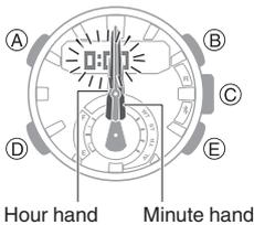
7. If the hour hand and minute hand are not at 12 o'clock, use (B) and (E) to align them.
