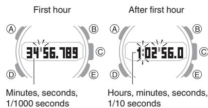
3. Press (A) to reset the elapsed time to all zeros.
