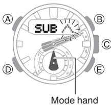
5. If the mode hand is not at 12 o'clock, use (B) and (E) to align it.
